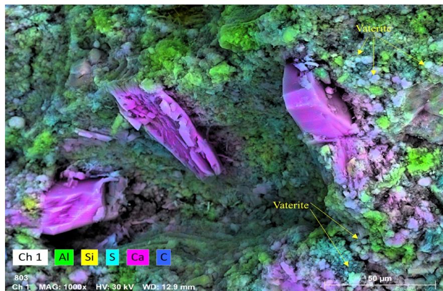
Fig. 19. SEM image of the VC3-15 mortar sample associated with elemental mapping by EDS at 3 days: (Al) aluminum, (Si) silicon, (S) sulfur, (Ca) calcium, and (C) carbon.
