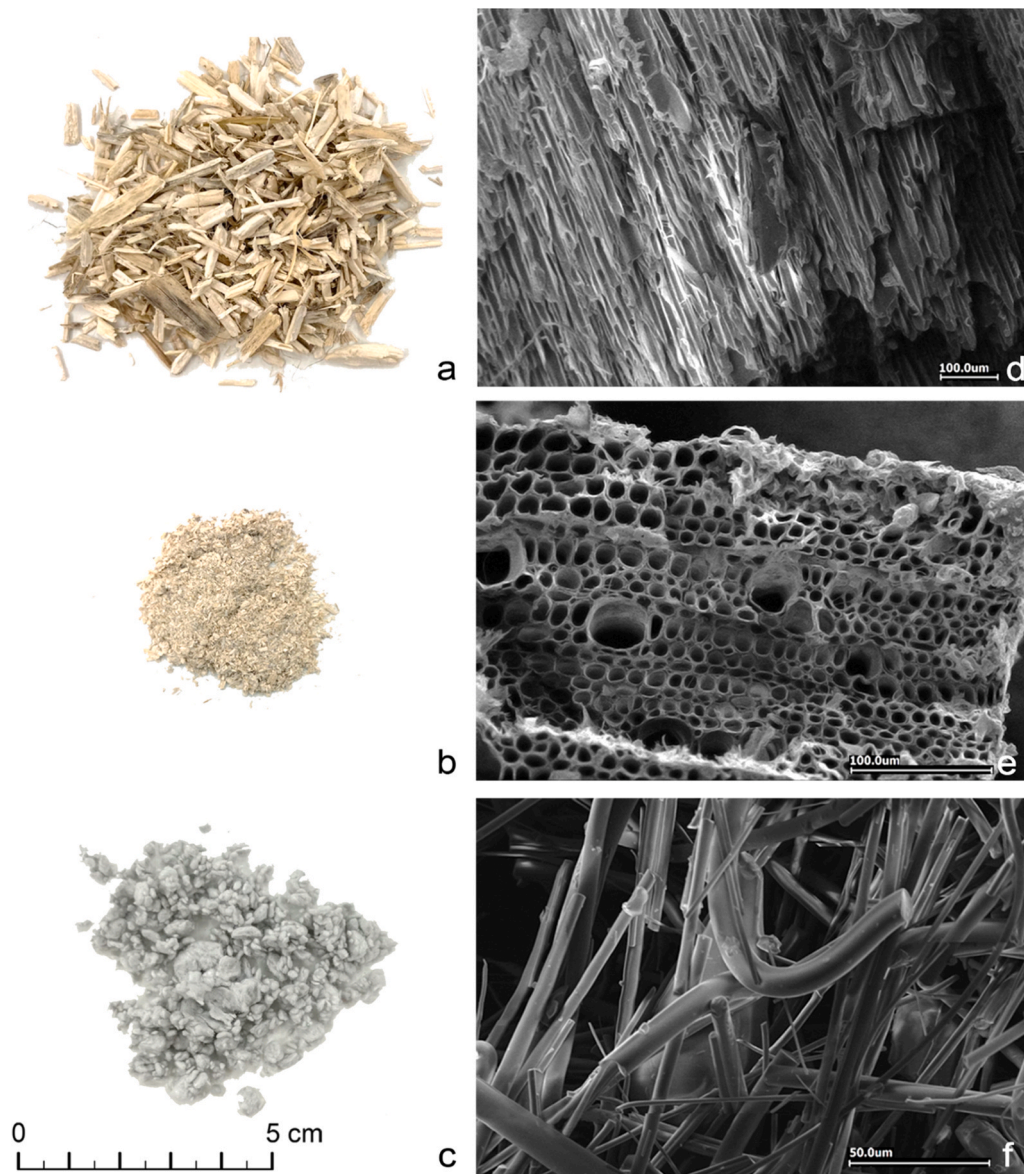
Fig. 3. Photographs of (a) raw hemp shiv, (b) ground hemp shiv, and (c) basalt fibre, along with SEM micrographs of the reinforcement materials showing (d) hemp shiv, (e) a cross-section of hemp shiv, and (f) basalt fibre.
