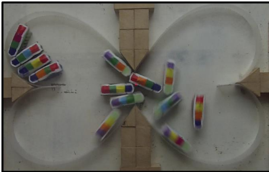
Figure 1: Experimental setup. Two regions are linked by a narrow opening. This particular geometry design allows to generate a continuous flow of agents between both regions.
