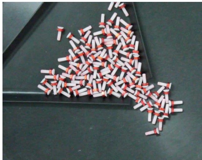
Figure 1: The figure shows an ensemble of screws passing a narrow gap of a funnel-shaped enclosure. The vibrating ground plate is tilted by about 1 deg towards the bottom-right corner. By video analysis, positions and orientations of all objects are detected and evaluated.
