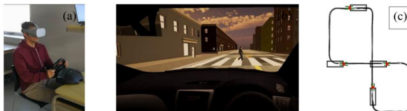
Fig. 1: scenario and system used for testing driving behavior in the presence of crosswalks in a VR environment. (a) VR system, (b) scenario screenshot and (c) selected car trajectory.
