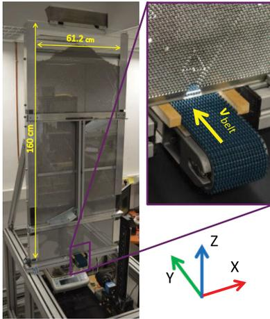
FIG. 1. Experimental setup. The close up shows the orifice region with the conveyor belt placed below. The yellow arrow indicates the belt direction of movement. The origin of coordinates system is set at the center of the orifice.
