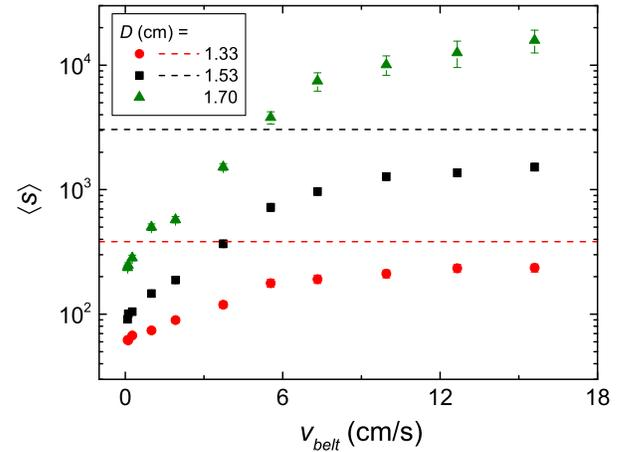
FIG. 2. Experimental data of the mean avalanche size as function of the belt velocity for the three outlet sizes indicated in the legend. In all cases we use spheres of diameter  $d_p = 4$  mm and a gap between the belt and the silo of  $h = 3.2 \pm 0.1$  mm. The horizontal lines correspond to the case where the silos are discharged only by gravity (without conveyor belt). Note the logarithmic scale in the y axis.
