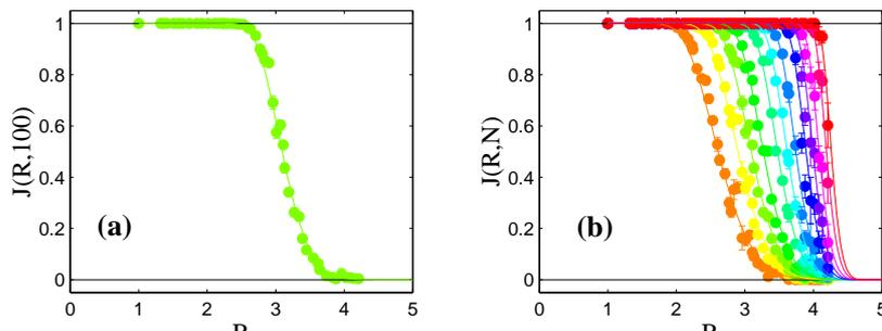
**Fig. 4.** The jamming probability  $J$  as a function of  $R$ . (a)  $J(R)$  for  $N = 100$ . (b)  $J(R)$  for  $N = 20, 50, 100, 200, 500, 1000, 2000, 5000, 10000, 20000, 50000, 100000$  (color changes from orange to red as  $N$  increases). The solid lines are the fits given by (6)
