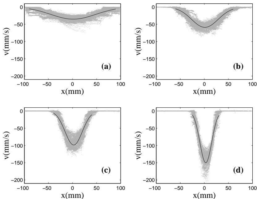
**Fig. 9.** Vertical velocity profiles inside the silo at different heights: (a)  $y = 355$  mm; (b)  $y = 155$  mm; (c)  $y = 65$  mm; (d)  $y = 30$  mm. All the plots are at the same scale. Solid lines are fits using (12). The diameter of the orifice is  $D = 15.8$  mm and the diameter of the beads is  $\phi = 1$  mm.
