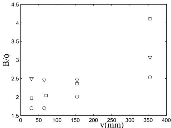
**Fig. 10.** The value of the parameter  $B$  (divided by the bead diameter to make it dimensionless) as a function of the height for three different orifice sizes:  $R = 4.8$  (squares),  $R = 9.5$  (circles) and  $R = 15.8$  (triangles)
