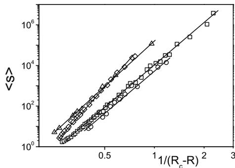
**Fig. 5.** The dependency of the mean avalanche size  $\langle s \rangle$  on  $R$  for rice (*triangles*), lentils (*diamonds*), spherical glass beads (*squares*) and irregular pasta grains (*circles*)
