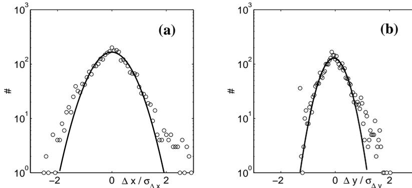
**Fig. 12.** The histogram for the fluctuations of the particle positions. They correspond to the fluctuations in the horizontal coordinate **(a)** and the vertical coordinate **(b)**, for  $R = 15.9$ . They are at the same scale and normalized by the standard deviation. The solid lines are the gaussian best fits
