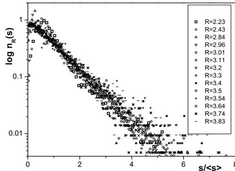
**Fig. 3.** Normalized histogram for a series of openings  $R$  as indicated in the legend, in semilogarithmic scale. The rescaling has been performed dividing in each histogram the avalanche size  $s$  by the mean avalanche  $\langle s \rangle$  corresponding to that particular  $R$
