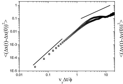
**Fig. 11.** Mean square displacements for  $R = 16$  as a function of time (note that time has been rescaled, so that one corresponds to the time it takes for a bead to fall a distance equal to its own diameter). The mean square displacements for the vertical direction (*squares*) and for the horizontal direction (*circles*) both show a ballistic behavior at short time scales and a diffusive behavior at long time scales (the solid lines have slopes 2 and 1)
