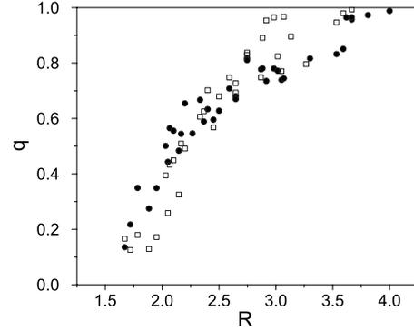
FIG. 6. Probability  $q$  that a blocking arch is destabilized due to the vertical vibration as a function of the opening size  $R$ . Results obtained with the probabilistic model, in which  $p$  does not depend on  $\Gamma$  (solid circles). Results obtained from the analysis of the weak jams (open squares). The data correspond to several sets of experiments; for some of them both methods were implemented, while for others only one of the measurements was performed.
