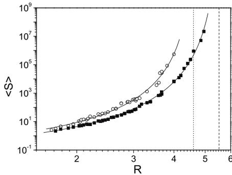
FIG. 5. Mean avalanche  $\langle s \rangle$  versus the dimensionless radius  $R$  for the vibrated ( $\circ$ ) and nonvibrated ( $\blacksquare$ ) silo. The solid lines correspond to fits using Eq. (1) with the parameters given in the text. The dotted line and the dashed line correspond to the values of  $R_c$  used in the fits.
