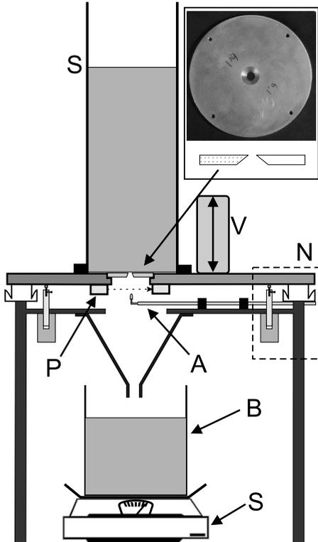
FIG. 1. Experimental device. S: silo; V: pneumatic vibrator; N: damping and isolation system (air cushions and valves); P: photo-sensor; A: compressed air duct; B: box; S: scales. The inset shows a photograph (from the bottom) and a sketch of the cross section of the changeable part in which the hole is bored.
