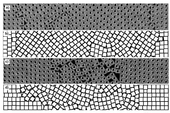
Fig. 2. Packings of square nuts and simulated particles with d = 1. Pictures of the experiment (a) after the silo filling and (c) after the partial discharge. Numerical graphs (b) and (d) on the same order.
