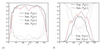
Fig. 4. Experimental and numerical orientation of the squares for different sectors of the silo a) at the end of the silo filling and b) after the silo partial discharge.  $P_{\frac{\pi}{2}}(x)$  accounts for the fraction of particles aligned mostly transversally to gravity, while  $P_{\frac{\pi}{4}}(x)$  accounts for the fraction of particles mostly aligned with gravity.
