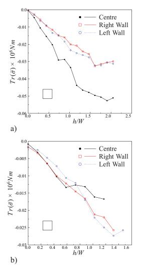
Fig. 8. Profiles of the trace of the mean stress tensor (pressure) after the load a) and the partial discharge b) for squares. In all cases the depth h is expressed in units of the silo width.
