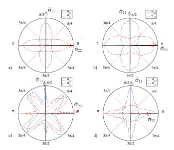
Fig. 5. (Color online) Polar distribution of the principal directions of the *local stress* for elongated particles with aspect ratio d = 5.4 (a) after the silo load and (b) after the partial discharge. The same results for squares (c) after the load and (d) after the partial discharge.
