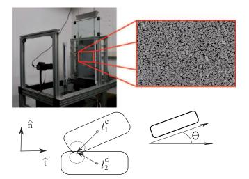
Fig. 1. Photograph of the experimental setup of the twodimensional silo. On the right, as example, there is a zoom of the d = 5.4 rods deposited in the bulk of the granular layer.
