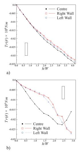
Fig. 7. Profiles of the trace of the mean stress tensor (pressure) after the load a) and the partial discharge b) for rods with d = 5.4. In all cases the depth h is expressed in units of the silo width.
