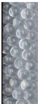
Figure 5. Helical arrangement of glass beads formed spontaneously inside the pipe.
