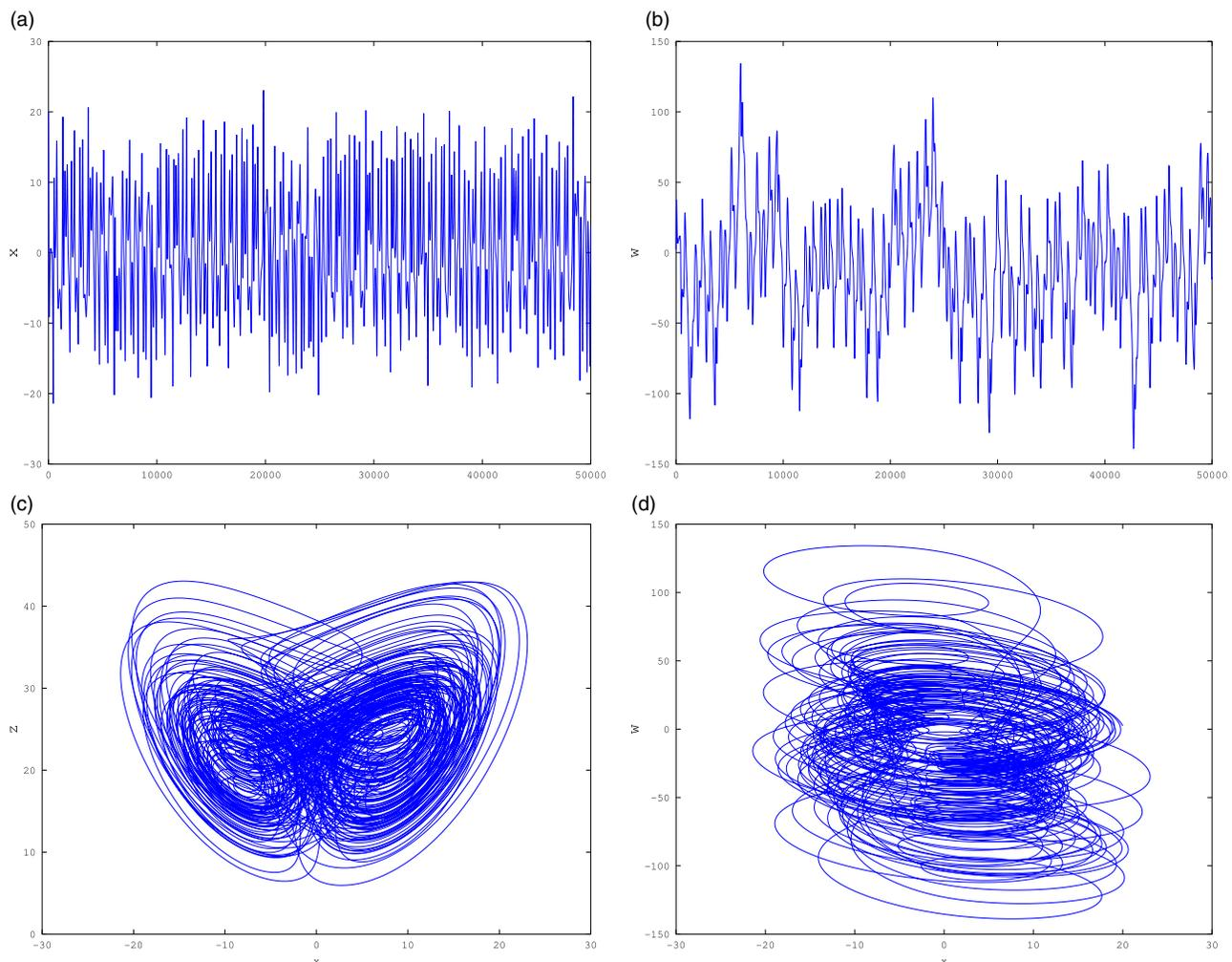
FIG. 3. Times series and phase space for Lü System under different variables and planes. (a) Time series for  $x(t)$  variable. (b) Time series for  $w(t)$  variable. (c) Phase space for the plane  $(x-z)$ . (d) Phase space for the plane  $(x-w)$ .
