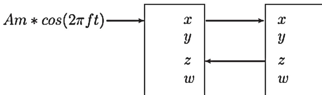
FIG. 1. Scheme of how dynamical systems are coupled and perturbed by a harmonic signal at frequency  $f$ .
