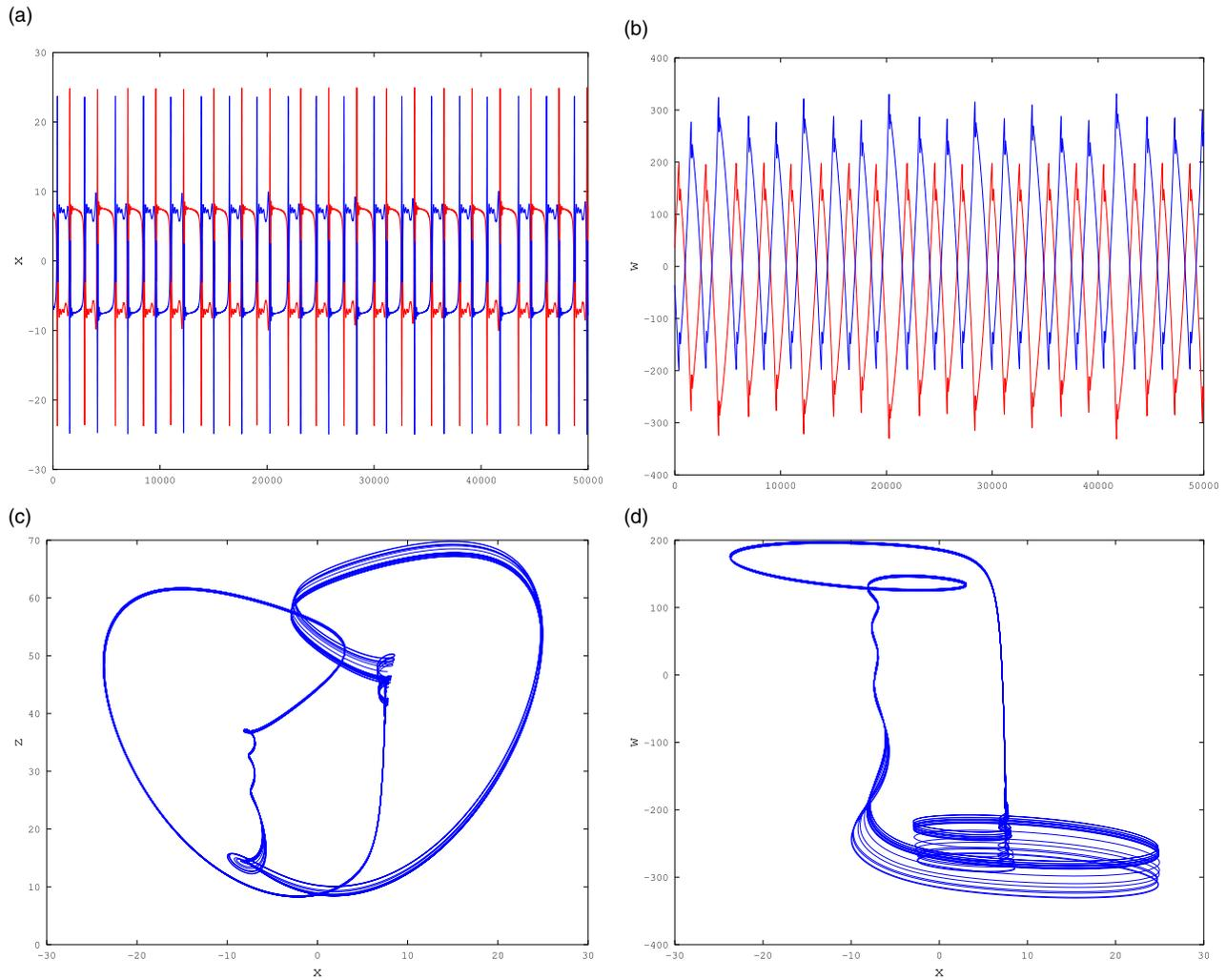
FIG. 5. Time series and phase space under different planes and variables for Lü coupled system. (a) Time series for  $x(t)$  variable for systems 1 and 2: blue for  $x_1(t)$ , whereas red for  $x_2(t)$ . (b) Time series for  $w(t)$  variable for systems 1 and 2: blue for  $w_1(t)$ , whereas red for  $w_2(t)$ . (c) Phase space for the projection  $(x-z)$ . (d) Phase space for the projection  $(x-w)$ .
