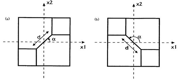
FIG. 2. Schematic representation of the asymmetric patterns, where  $d$  stands for the length of the diagonal segment and  $\alpha$  is the angle between that segment and the  $X_1$  axis. In our experiment  $\alpha = \pi/4$  or  $3\pi/4$ . The variable  $x$  defined in Eq. (1) is thus positive in (a) and negative in (b). A symmetric pattern would be characterized by  $x = 0$ .
