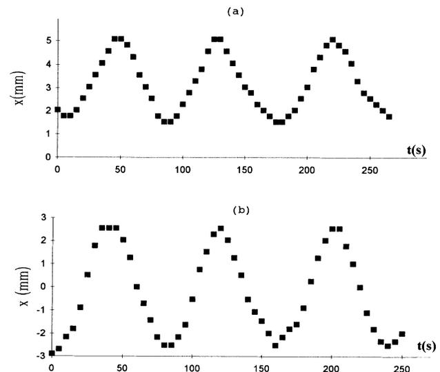
FIG. 3. Pieces of the time series data giving the evolution of the variable  $x$  as a function of time. The error in the  $x$  values (measured using an image processing code) is of about 0.2 mm. (a) shows a periodic modulation of  $x$  for a pattern similar to the one in Fig. 1(a) (aspect ratio  $\Gamma = 4.46$ , temperature  $T = 57^\circ\text{C}$ ). (b) shows a periodic alternation between the two asymmetric patterns 1(a) and 1(c) ( $\Gamma = 4.46, T = 59.8^\circ\text{C}$ ).
