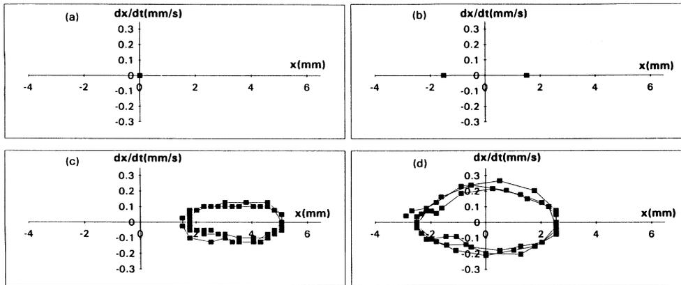
FIG. 4. Reconstructed phase space  $(x, x')$ . In (a) a fixed point in  $(0,0)$  corresponding to a stationary symmetric pattern ( $\Gamma=4.46, T=35^\circ\text{C}$ ). (b) shows the fixed points corresponding to the stationary asymmetric patterns ( $\Gamma=4.46, T=45.6^\circ\text{C}$ ). In (c) and (d) we display the phase space embeddings of the data presented in Fig. 3. The derivative was computed for the  $n$ th point as  $(x_{n+1} - x_{n-1})/2\delta t$ .
