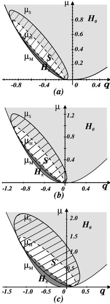
FIG. 3. Stability diagrams taking into account spatial quadratic terms. Parameter values: (a)  $A\eta=0.8$ ,  $\alpha_1=0.22$ ,  $\alpha_2=-2.4 \times 10^{-4}$ ; (b)  $A\eta=0.92$ ,  $\alpha_1=0.22$ ,  $\alpha_2=-1.3 \times 10^{-4}$ ; (c)  $A\eta=1.59$ ,  $\alpha_1=0.21$ ,  $\alpha_2=-2.7 \times 10^{-3}$ .
