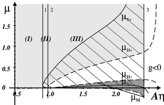
FIG. 2. Stability thresholds in the parameter space  $(A\eta, \mu)$  for Turing patterns. Shaded and striped regions denote stable hexagons and bands, respectively. In region I only hexagons are stable. Hexagons and bands coexist for  $\mu_{S-} < \mu < \mu_{H-}$  in region II. In region III hexagons are unstable within the range  $\mu_{H+} < \mu < \mu_{S+}$ . To the right of line 3,  $g < 0$  and, therefore, terms higher than cubic are needed in the amplitude equation.
