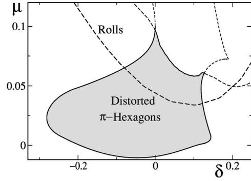
FIG. 4. Amplitude stability zone for squeezed hexagons (shaded region). Above the lower dashed line, stripes are also stable. Parameter values:  $A\eta=1.59$ ,  $\alpha_1=0.21$ ,  $\alpha_2=-2.7 \times 10^{-3}$ .
