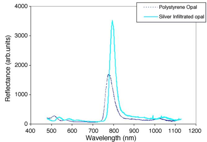
Fig. 4. Reflectance measurement of non-infiltrated and silver-infiltrated opals. Incidence angle is 45°.
