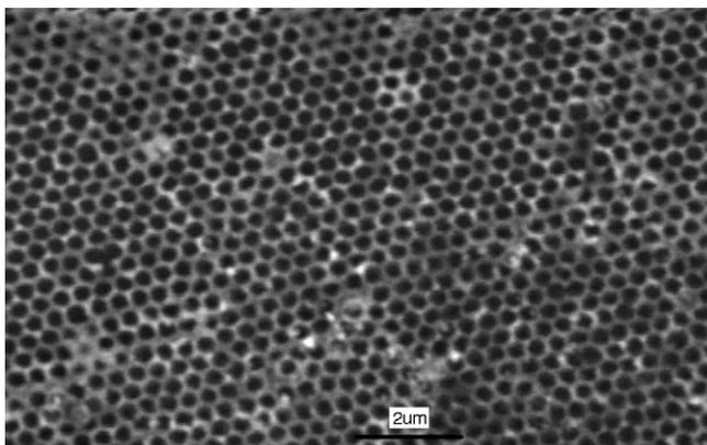
Fig. 3. Nanostructured silver after removal of the polystyrene spheres with toluene.
