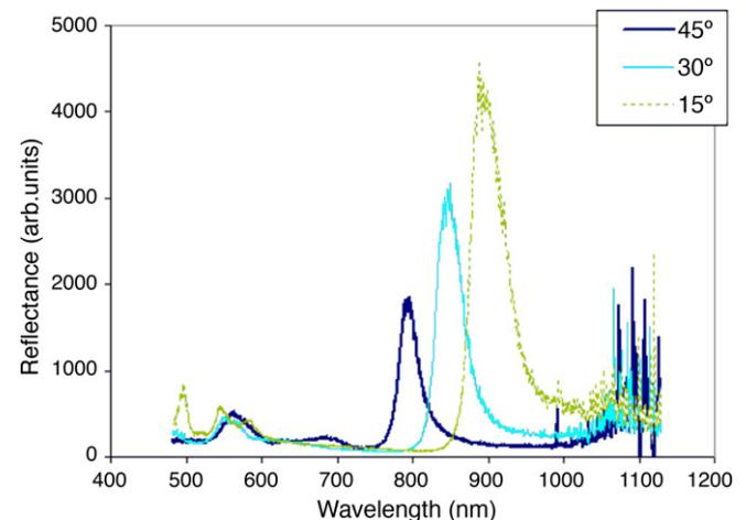
Fig. 5. Reflectance measurements of non-infiltrated polystyrene opals with incident angles of 15°, 30° and 45°.
