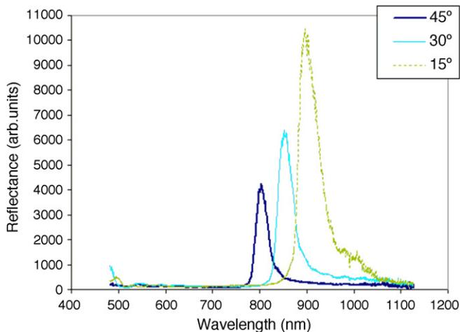
Fig. 6. Reflectance measurements of silver-infiltrated polystyrene opals with incident angles of 15°, 30° and 45°.
