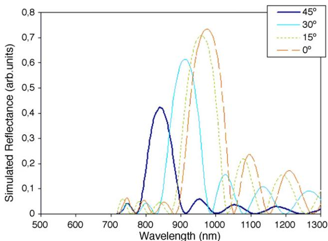
Fig. 7. Theoretical simulations of the reflectance of polystyrene opals with incident angles of 15°, 30° and 45°.
