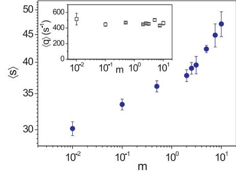
FIG. 3. (Color online) Logarithmic plot of the mean avalanche size vs the mass of the particles obtained for  $\Gamma = 1$ . Inset: lin-log plot of the flow rate, in number of particles per second, for  $\Gamma = 1$  and different values of the mass of the particles.
