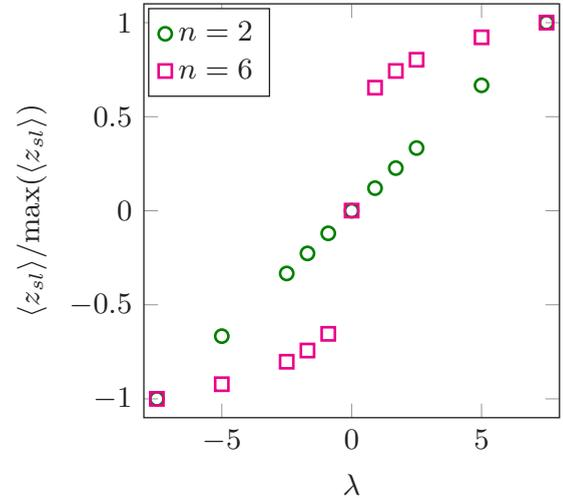
FIG. 8. Evolution of the shear layer position with  $\lambda$  for different  $n$  and  $\sigma = 0.1$ . The normalization is made using the maximal  $z$  in the explored range of  $\lambda$ .
