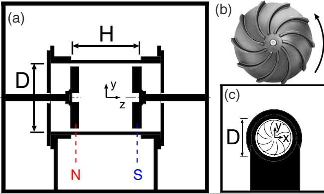
FIG. 1. Global scheme of the experimental setup. (a) Side view of the cavity with the denomination of the propellers; (b) photograph of a propeller with its rotation direction; (c) side view of the cavity in the propeller's axis direction.
