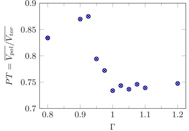
FIG. 6. Poloidal-toroidal ratio in the flow vs the aspect ratio for  $\Delta \cong 0$  and  $Re = 2.9 \times 10^5$ .
