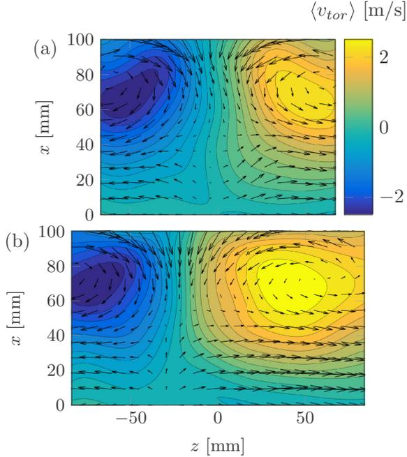
FIG. 5. Overlaid contour plots of the mean toroidal velocity  $v_{eq}$  and the mean vector plots of the poloidal velocity  $(v_z, v_r)$  between the propellers blades extremities and  $y \in [0, R]$  for (a)  $\Gamma = 0.9$  and (b)  $\Gamma = 1.075$ . The color bar is shared by both figures.
