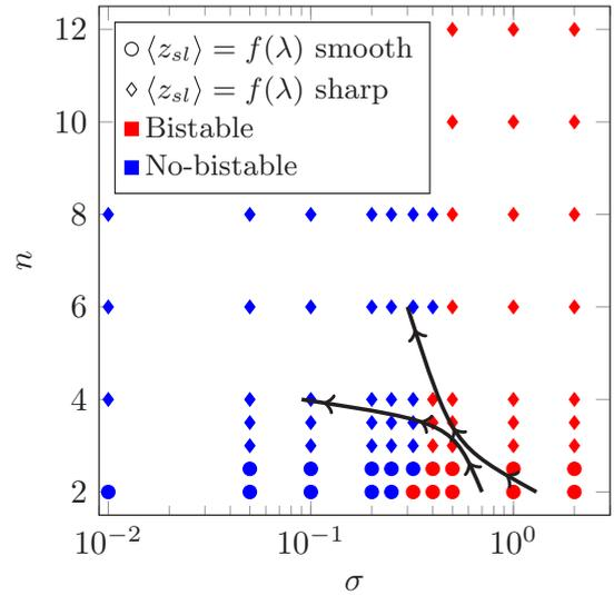
FIG. 9. Phase diagram of the shear layer behavior based on the Langevin equation with colored noise equation for  $B_0 = 1$  and  $\tau_p = 1$ . The black arrows are possible trajectories in the phase diagram when  $\Gamma$  is increased.
