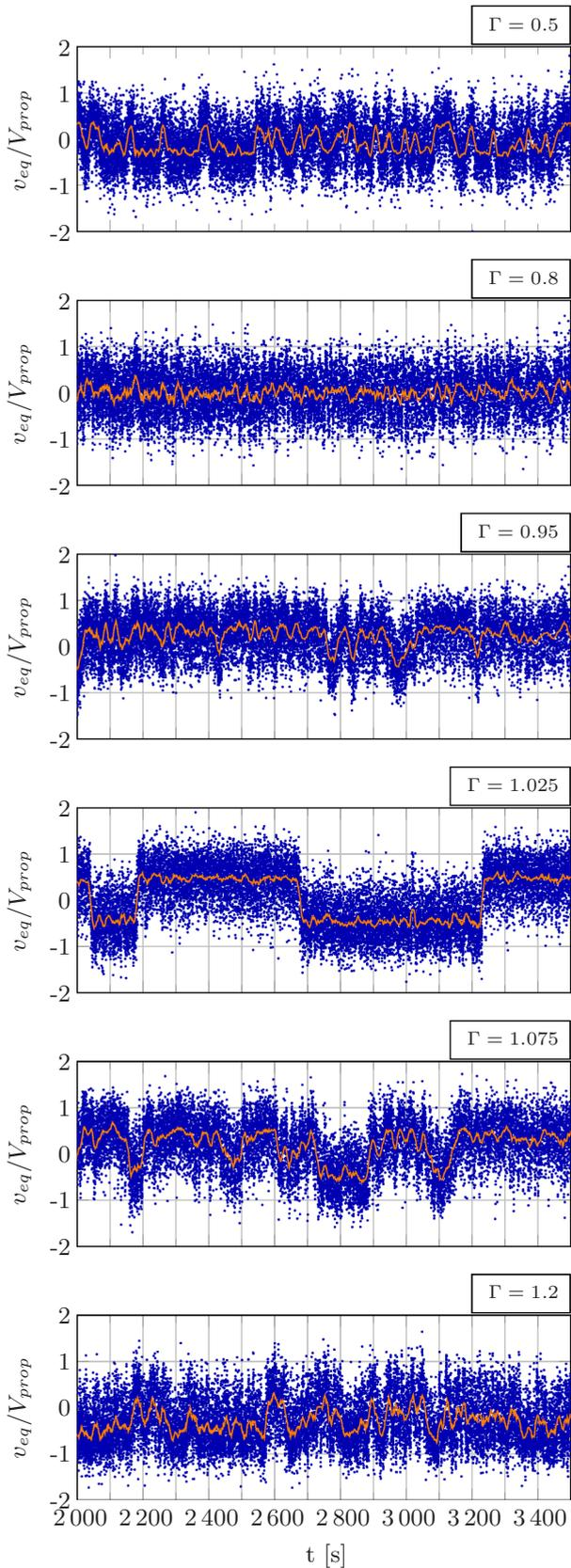
FIG. 2. Time series of the equatorial velocity at ( $z=0, y=0.9 R$ ) for six different aspect ratio.  $V_{prop}$  represents the velocity of the propellers at the blades outlet. The orange solid lines represent the sliding mean value of the velocity signal.  $Re = 2.9 \times 10^5$  and  $\Delta \cong 0$ .
