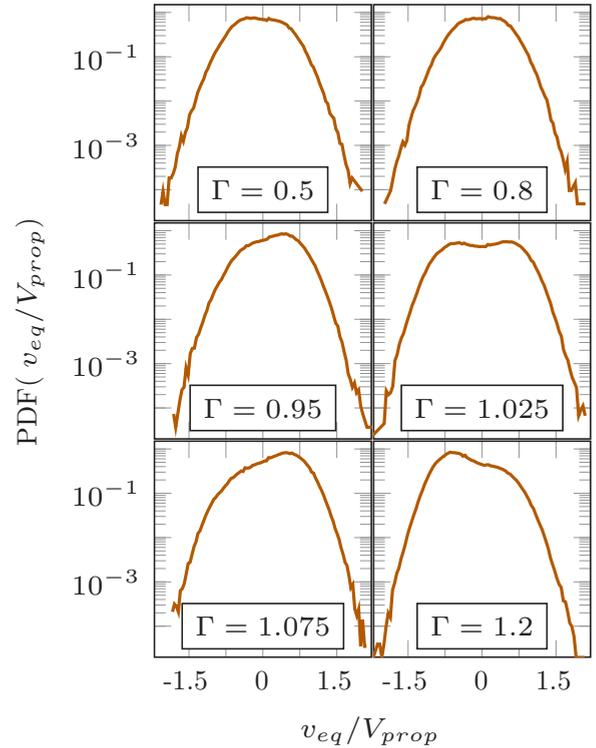
FIG. 3. Probability density functions of the normalized velocity for six different aspect ratios. They correspond to the time series presented on Fig. 2.
