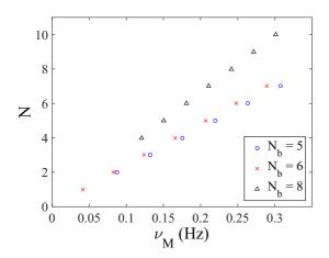
FIG. 2. (Color online) Number of streaks (N) developed for different modulation frequencies  $(v_M)$ . Results, obtained with a half-filled drum, are presented for base patterns with different number of streaks  $N_b$  (and hence different  $\omega$ ) as indicated in the legend.
