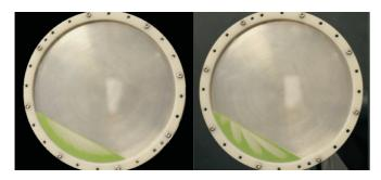
FIG. 7. (Color online) A filling fraction of 10% with steady rotation of  $\omega = 0.095$  rad/s (left) and exhibiting four streaks after modulation with  $\nu_M = 0.0045$  rad/s (right).
