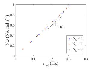
FIG. 3. (Color online) Number of streaks multiplied by the constant rotation frequency ( $\omega$ ) for different modulation frequencies and a filling fraction of 50%. A linear fit of the results gives a relationship  $N\omega = (3.16 \pm 0.08)v_M$ . As in Fig. 2, we present results obtained with a half-filled drum with different number of streaks in the base pattern  $N_b$  (and hence different  $\omega$ ) as indicated in the legend.
