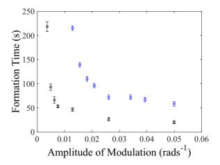
FIG. 8. (Color online) The time taken for a transition from six petals base pattern to five petals pattern measured as a function of the amplitude of the modulation for  $f_f = 50\%$  (o) and  $f_f = 20\%$  ( $\square$ ). The finite amplitude below which the transition was not observed to occur, even after time periods of  $\sim$ 24 h, can be seen to increase with increased filling fraction.
