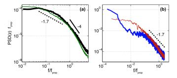
FIG. 3. (a) Power spectrum densities (noted PSD) of the axial position z for 6 mm (thin solid line) and 18 mm (thick solid line) particles in the S-vK with  $f_{\text{prop}} = 3$  Hz. (b) PSD of z for 10 mm (thin solid line) and 30 mm (thick solid line) particles in the C-vK with  $f_{\text{prop}} = 3.16$  Hz.
