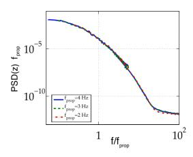
FIG. 4. Normalized spectra  $f_{\text{prop}}\text{PSD}(z)$  of the axial position z for 6 mm particles, plotted as a function of the reduced frequency  $f/f_{\text{prop}}$ , measured for three rotating frequencies  $f_{\text{prop}} = 2,3,4$  Hz in the S-vK setup.  $f_{\text{prop}} = 4$  Hz (solid line),  $f_{\text{prop}} = 3$  Hz (dashed line), and  $f_{\text{prop}} = 2$  Hz (dashed-dotted line).
